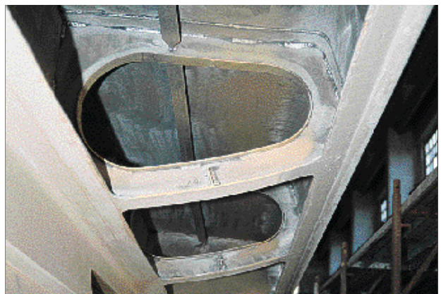
Building and assembly time can be reduced by using standard extrusions.
