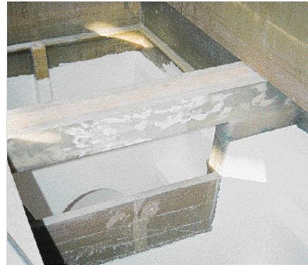
Integral tanks can be built in composites hulls.
