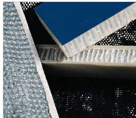
Tubulam is a honeycomb with cylindral cells. It has a wide range of applications.
