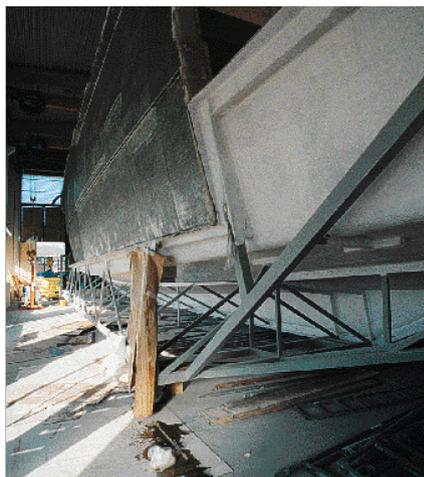
The hull bottom laminate is molded on a male mold while the topsides have fabricated on temporary female molds.
