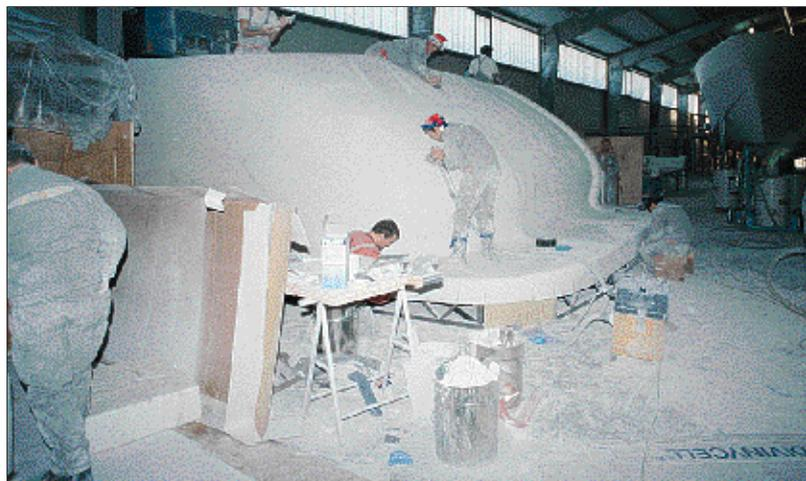
mize the tooling costs, the hulls are generally built on a **plug** or male mold made out of wood strips or plywood depending on the complexity of the shapes. The high performance hulls are built with sandwich composites using high properties cores, fibers and resins. Some builders have been using low temperature **prepregs with post curing** to improve the properties. Only a few builders have the know how and can afford the equipment to use this method of construction.
