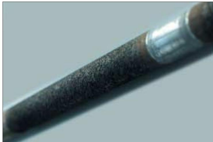
This propeller shaft suffered from DC stray current corrosion.
