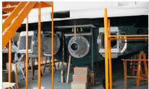
Two directional waterjets and one fixed power waterjet at center.
