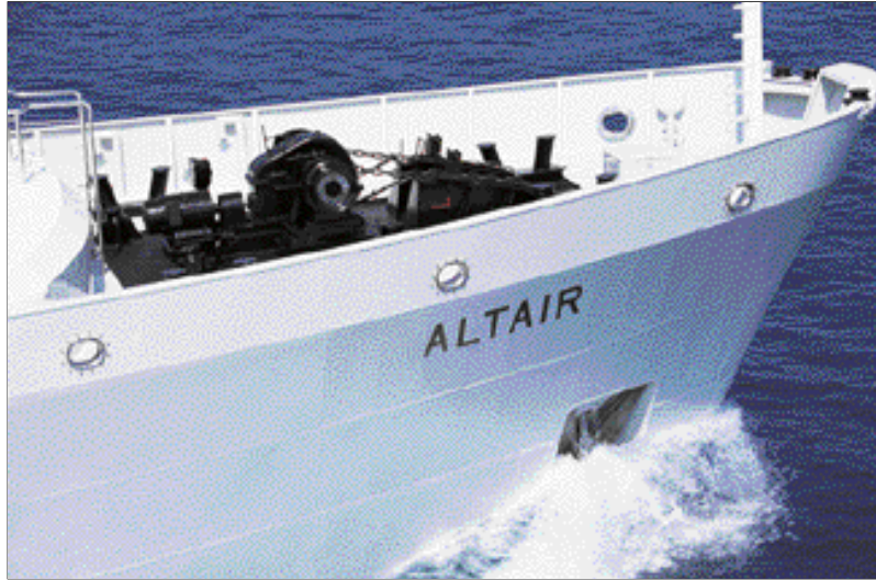
The original anchor windlasses were preserved onboard Altair.
