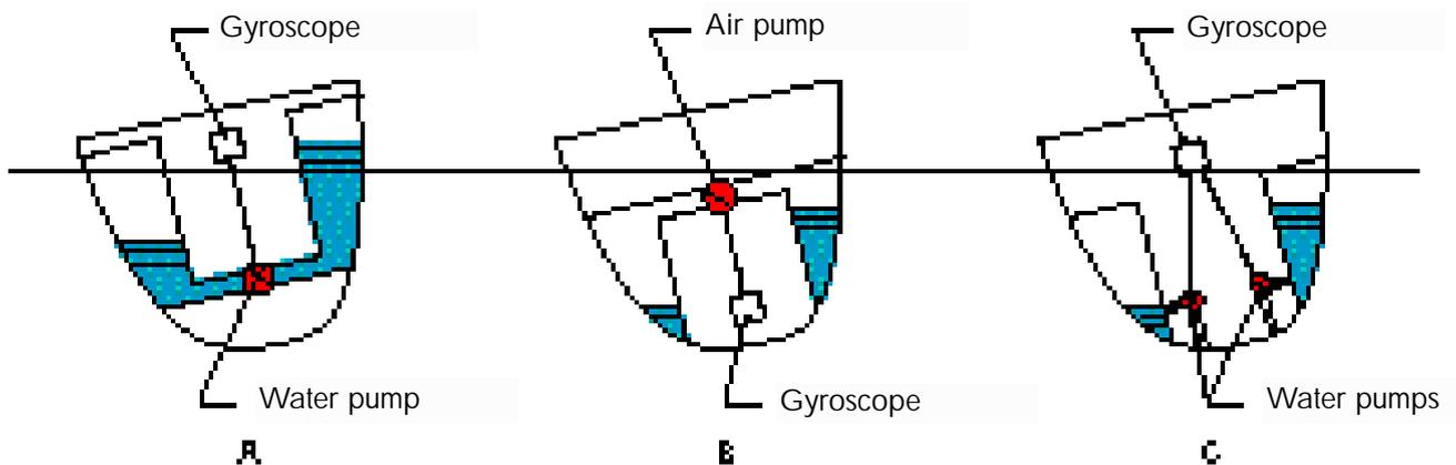
Three types of anti-roll tanks of the active type, with a roll sensor, water and air pumps.
