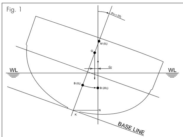
Position of the various centers of an inclined hull.
